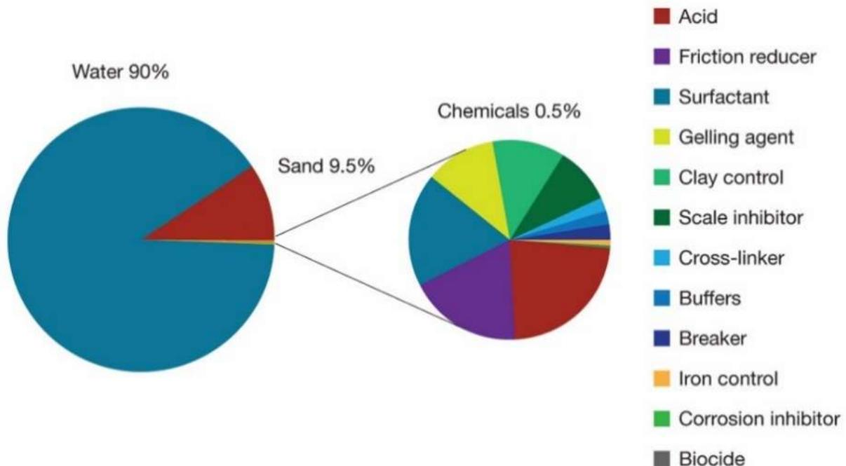
**Figure 3.** The make-up of typical hydraulic fracture stimulation fluid. Source: Department of Mines, Industry Regulation and Safety, WA.
