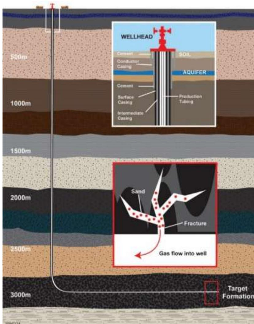
**Figure 1.** Schematic diagram showing a horizontal well intersecting a shale formation, in a typical Western Australian setting. At the surface, hydraulic fracture stimulation equipment (including the frack tree) is attached to the Christmas tree on top of the well. The horizontal section has undergone hydraulic fracture stimulation. Lower inset shows induced fractures in the shale formation. Source: Department of Mines, Industry Regulation and Safety, WA.
